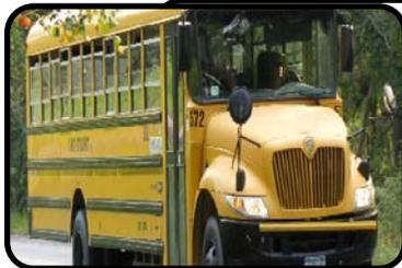
A **Type "C"** school bus is constructed utilizing a chassis with a hood and front fender assembly. The entrance door is behind the front wheels.
