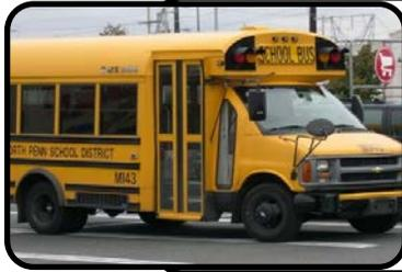
A **Type "A"** school bus is a van conversion or bus constructed utilizing a cutaway front-section vehicle with a left side driver's door. The entrance door is behind the front wheels. The definition includes two classifications:
