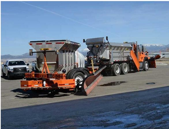
The Tow Plow is a steerable trailer-mounted plow that is pulled behind a plow truck. The Tow Plow can be rotated to one side of the truck, which doubles the plow width. The 26-foot-wide plow gives the operator the ability to move snow from two lanes of roadway in one pass.
