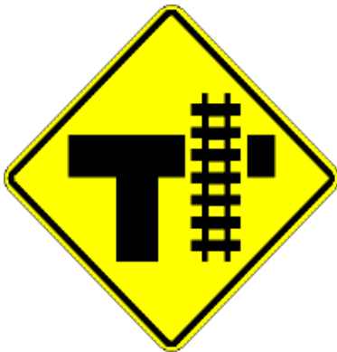
Parallel Railroad Crossing - T
